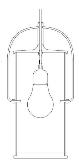
Thanks to the simplicity of its conception Elio is ready for industrialization. This is a smart product that makes a strong effect but is not technically complex. The top part and the diffuser can be attached thanks to the metallic branches that are inserted into small wholes in the diffuser
